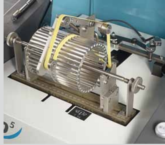
Belt drive from above for balancing of radial fans
