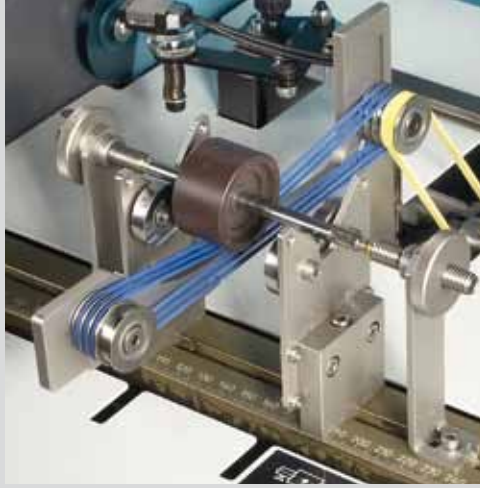
Balancing of permanent magnet armatures with 3 drive belts
