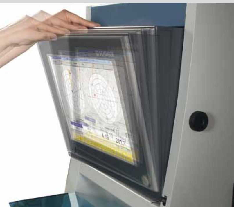
The adjustable viewing angle of the measuring unit screen enables glare free working.
