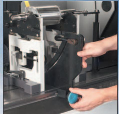
The belt drive can be adjusted to the correct rotor diameter in no time.
