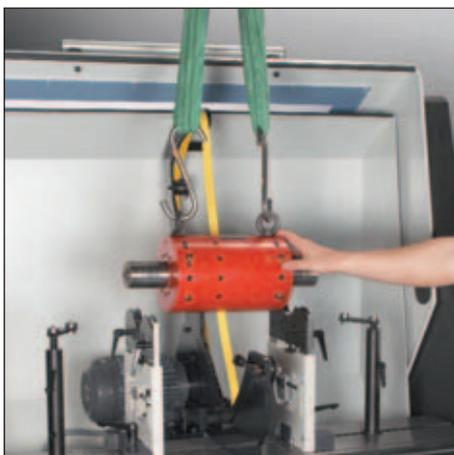
Rotors can be loaded easily from above using a crane. Compact in its outer dimensions, yet lots of room for large rotors.
