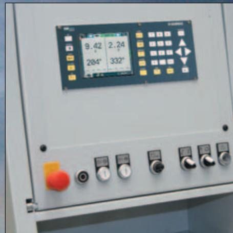
CAB 700 is universal and cost efficient basic measuring instrument for all standard balancing tasks.
